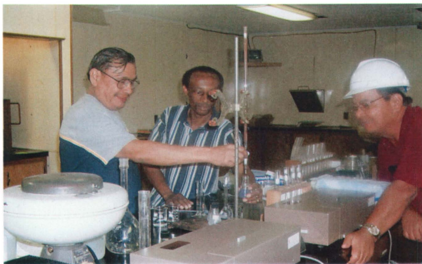
Figure 6.3. Photograph of the use of the Eggleston (14) titration method to measure the activity of commercial dextranases at the factory
